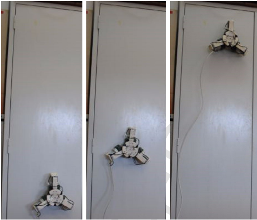
Fig. 19. A laboratory experiment on a flat surface of a locker. The omniclember could successfully navigate on the locker, which is made of a very thin steel sheet less than 1mm .
