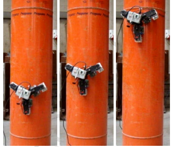
Fig. 20. Omniclember tested on the 150mm radius propane bottle.
