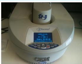
Figura 12: Digestor CEM modelo Discover® SP-D
