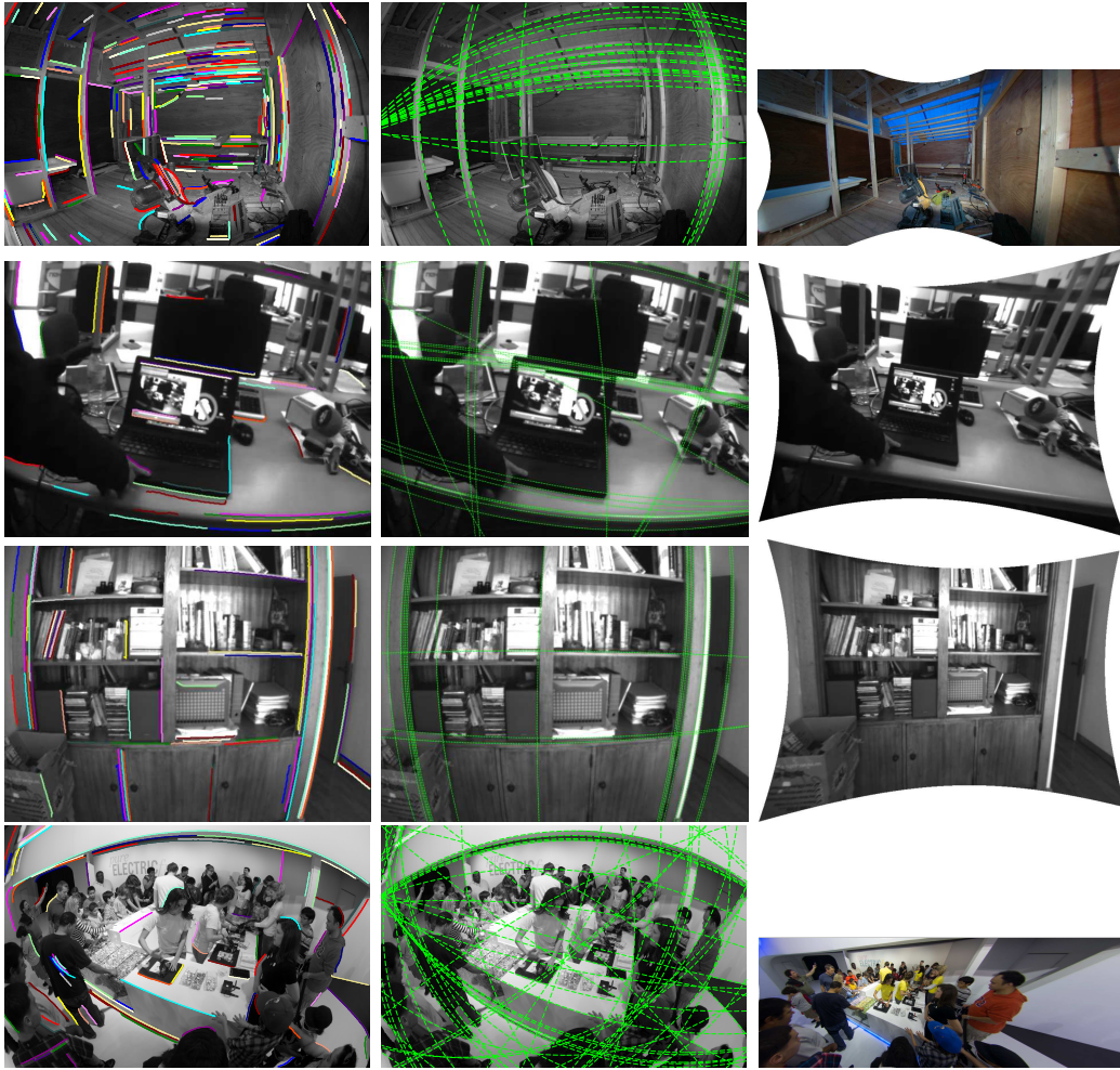
Figure A.3: Results of the unsupervised plumb-line calibration. Data set # 3
