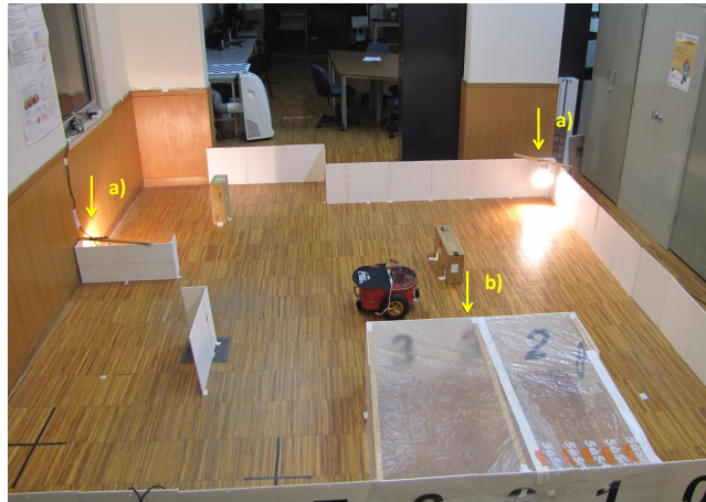
Figure 6.3: Real scenario with three points of interest for SVM classification. a) Fire outbreak emulated using a 500 watts spotlight. b) Contaminated enclosed area with alcohol.
