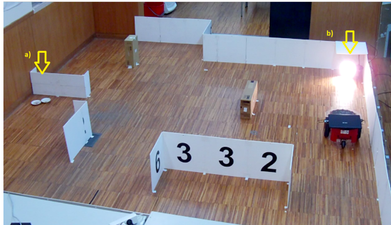
Figure 6.1: Real scenario with two points of interest for SVM classification. a) Contamination using alcohol and petrol; b) Fire outbreak emulated using a 500 watts spotlight.
