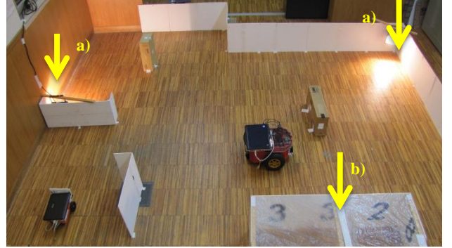
Figure 6. Real scenario with three point of interest for SVM classification. a) Fire outbreak emulated using a 500 watts spotlight. b) Contaminated enclosed area with alcohol.
