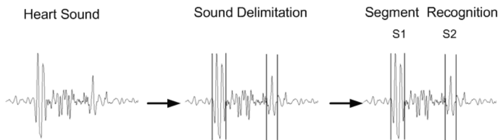
Figure 5.1. Main constituent blocks of heart sound segmentation. Delimitation determines onsets and offsets of the sounds which are addressed as segments or gates, and Recognition identifies the types of sounds.
