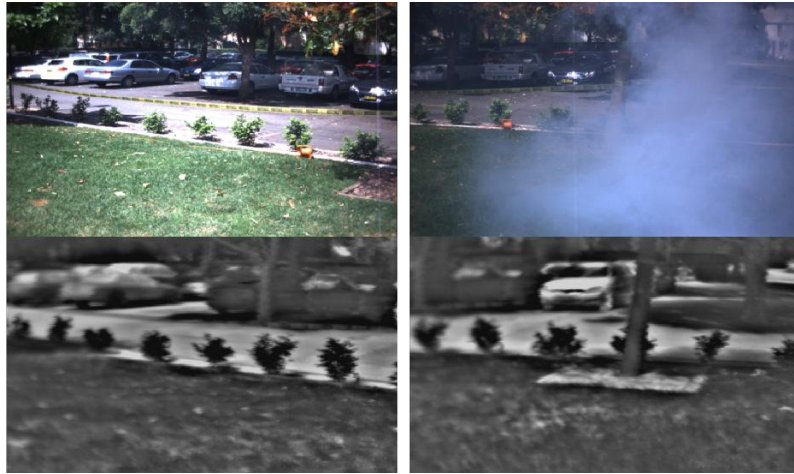
Figure 3.2: Representative images in clear conditions (left column) and in smoke (right) from the visual (top row) and thermal (bottom) cameras [BPVC12].
