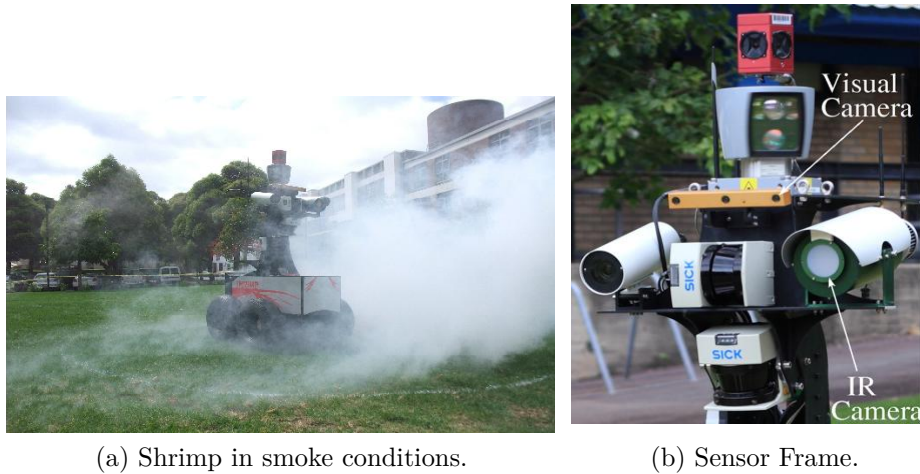
Figure 3.1: Experimental Setup [BPVC12].
