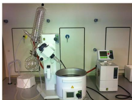
Figure 5.2 Buchi - Rotavapor R-210 with a vacuum pump V-700 and a vacuum controller V-850.
