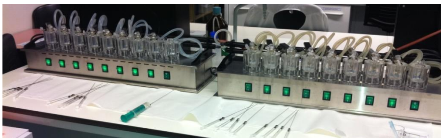
Figure 3.3 Franz diffusion cells (PermeGear, Inc., PA, USA) with a diffusion area of 0.64 cm 2 and a receptor compartment of 5.1 mL.
