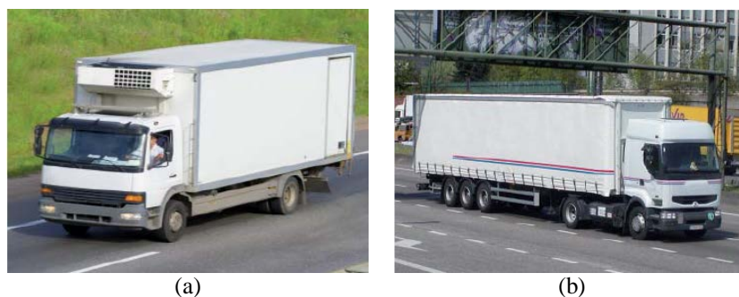
Figure 1.1 – Illustration of the trucks: (a) – lorry/truck and (b) – articulated vehicle (Eurostat et al., 2009)
