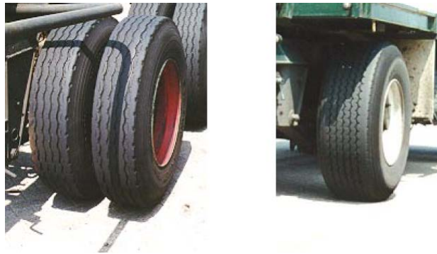
Figure 2.24 – Examples of dual tyre and wide base tyre (COST 334, 2001)
