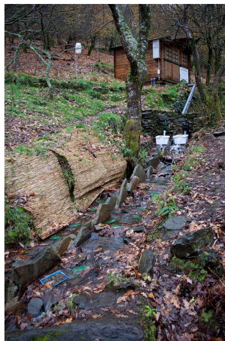
Fig. 1 Stream reach studied, showing the longitudinal schist division and the upstream dam with the two valves that provided water to each stream half. Pipes transported the water from two tanks (inside the wooden shelter on the stream bank) into the valves. The experimental stream half is on the left, and the control half is on the right of the schist division. Photo credit: João Rosa
