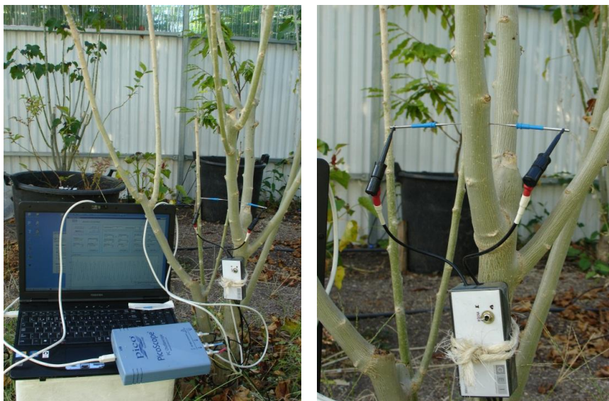
Figure 6.8: EIS measurement setup in the greenhouse.
