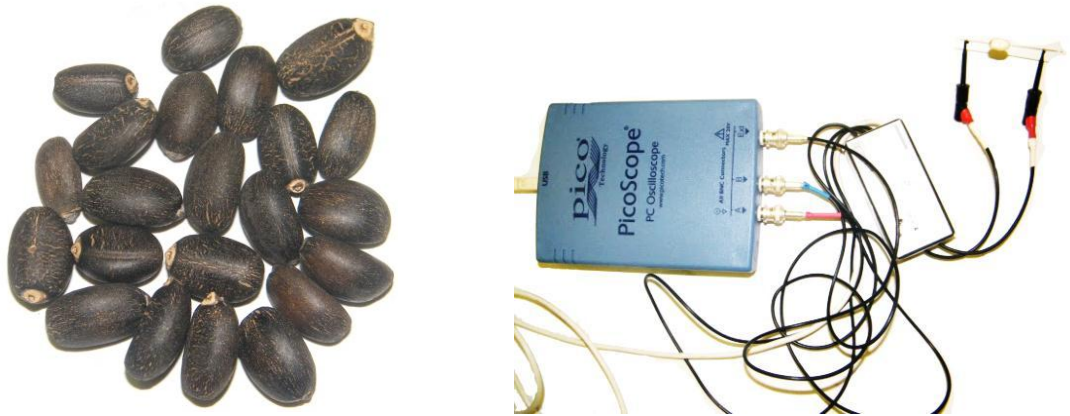
Figure 6.5: Jatropha seeds (left) and EIS system with Jatropha seed without shell (right).
