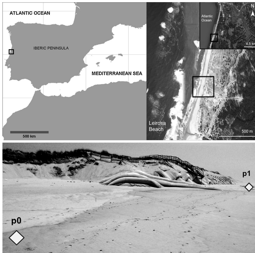
Fig. 1. (a) Study site: location of the Leirosa beach on the Portuguese coast ( 40^{\circ} 02' 57.33'' N, 08^{\circ} 53' 35.01'' W); photo credits for the image on the right: Google Earth, Version 6, accessed January 2012, adapted from Bessa et al. (2013b). (b) The experimental sites: p0 = shore in front of the natural dune, p1 = shore in front of the reconstructed dune, where the geotextile tubes are well visible (photo by D.H. Nourisson).
