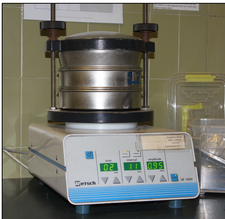
Figure 3 – Sieve shaker used to separate the sediment collected in Candal stream (< 2 mm) by size classes (< 2 mm and < 0.063 mm)
