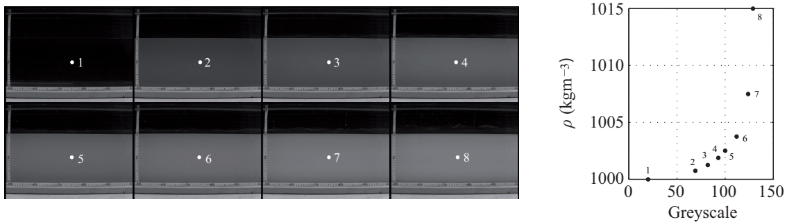
Figure 2.8: Example of images used for calibration and corresponding calibration curve. The reference point corresponds to one central pixel of the image and is represented in the frames by white dots
