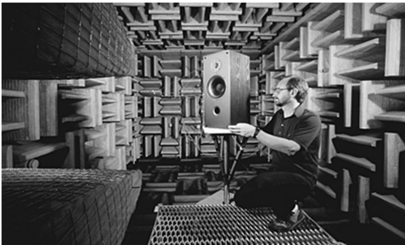
3. Exemplo de sala anecóica, National Research Council of Canada
