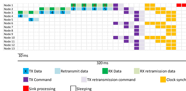
Figure 10.7 – TDMA schedule to meet the event latency
