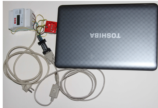
Figure 3.6.: Hardware used to collect the datasets: a smart meter, a laptop and the required converter. Apart from the laptop, the apparatus was supplied by ISA (ISA-Intelligent Sensing Anywhere, S. A., 2012).
