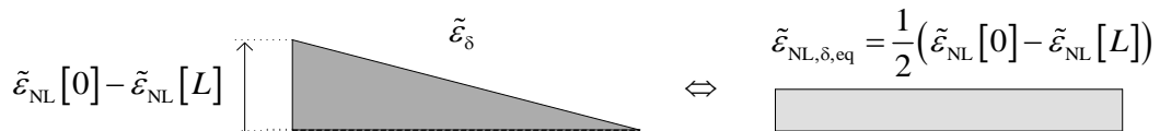
Figure 4.13. Equivalence between the fields \tilde{\varepsilon}_\delta and \tilde{\varepsilon}_{\delta,eq} in the context of the approximation of FFM(N) discrete description.
