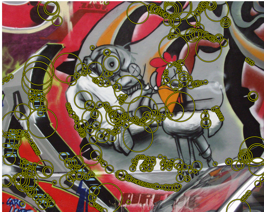
Figure 2.7: Feature extraction using the Laplacian of Gaussian.
