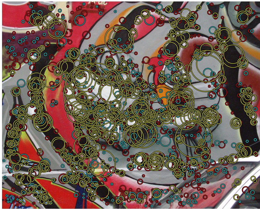
Figure 4.1: Combined feature detection: cyan circumferences enclose SFOP features when \alpha = 90^\circ ; red circumferences enclose SFOP features when \alpha = 0^\circ ; yellow circumferences denote the boundaries of Hessian-Laplace regions (blobs). Best viewed in color.
