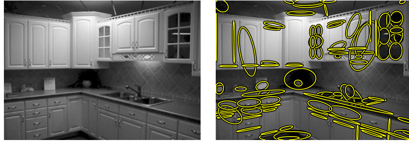
Figure 5.4: An example of MSER detection where most regions are anchored at objects boundaries. Left: input image; right: MSER detection
