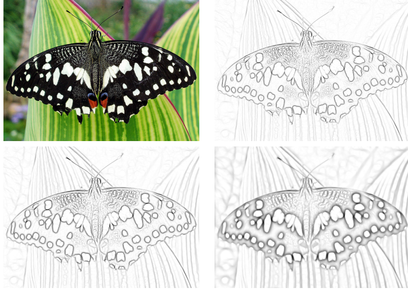
Figure 5.7: Proposed ridge highlighting: (a) input image; (b) principal curvature response; (c) ridge highlighting (4 scales); (d) ridge highlighting (12 scales). Darker structures in the saliency maps are the most salient ones. The parameters \sigma_0 and \xi were set to 1 and \sqrt[4]{2} , respectively.
