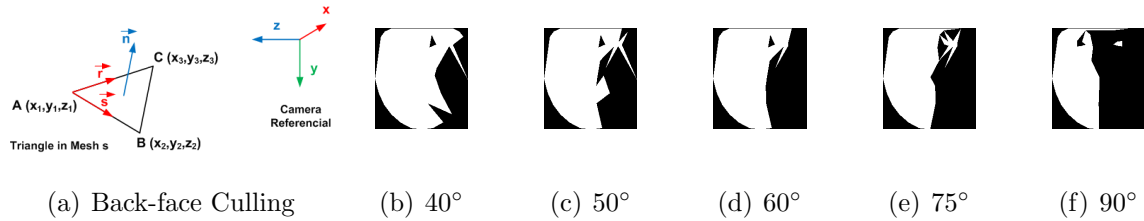
Figure 2.6: a) Back-face Culling illustration. \mathbf{n} is the normal vector from a triangle in mesh s and \mathbf{z} is the view vector from the camera reference. Images (b)(c)(d)(e) show the triangle visibility mask over the projected base mesh, s_{0\mathbf{p}} , for a head pan variation of 40^\circ , 50^\circ , 60^\circ , 75^\circ and 90^\circ w.r.t the base pose using the Back-face Culling technique. Non-visible triangles (in black) are not used to update the parameters.
