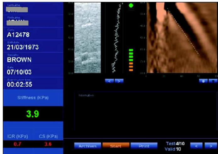
Figure 19. Measurement image for Transient Elastography. The result of 3.9 kPa indicates that the patient has an F0 fibrosis stage. Reproduced from www.jle.com/fr (“Le FibroScan®: un nouvel outil pour l’évaluation non invasive de la fibrose au cours des maladies chroniques du foie”).
