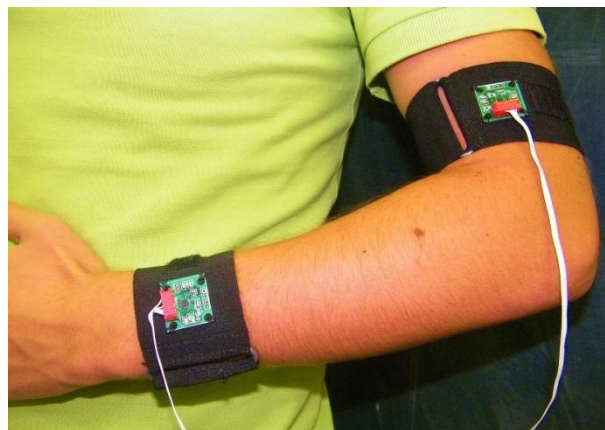
Figure 5.3 – Accelerometers are attached to a wristlet and an armband and placed in a stable manner in the subject forearm and arm.
