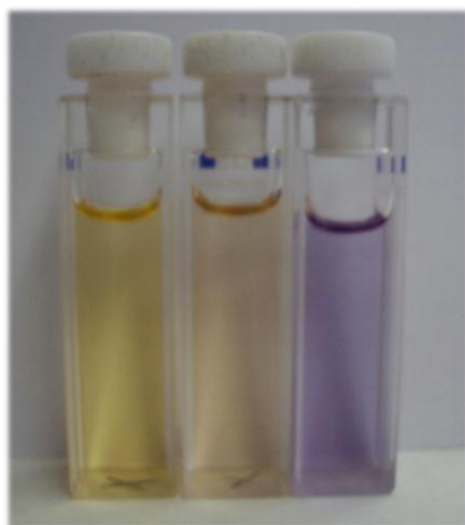
Figure 62 – Picture of Dracoflavylum dissolved in: DMF with some drops of HCl 1M (Yellow); neutral DMF (Orange); DMF with some drops of NaOH 1M (Purple blue).
