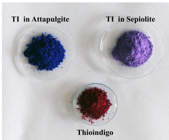
Figure 42- Photograph of thioindigo (down), and thioindigo mixed with attapulgite (top left) and sepiolite (top right), in a 20% proportion w/w.
