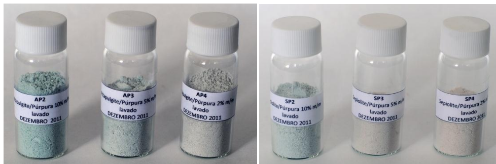
Figure 54 – Photograph of the different (weight/weight) mixtures dye/clay studied. Left: Tyrian purple/attapulgite, 10, 5 and 2% counting from the left. Right: Tyrian purple/sepiolite 10, 5 and 2% counting from the left.
