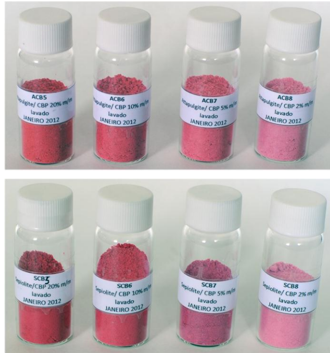
Figure 53 – Photograph of the different (weight/weight) mixtures dye/clay studied. Top: ciba brilliant pink/attapulgite, 20, 10, 5 and 2% counting from the left. Down: ciba brilliant pink/sepiolite, 20, 10, 5 and 2% counting from the left.
