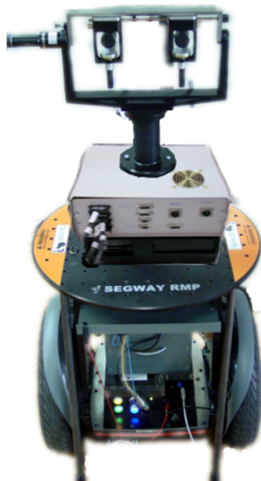
Figure 2.12: Four degrees of freedom robotic head mounted on Segway robotic platform body.
