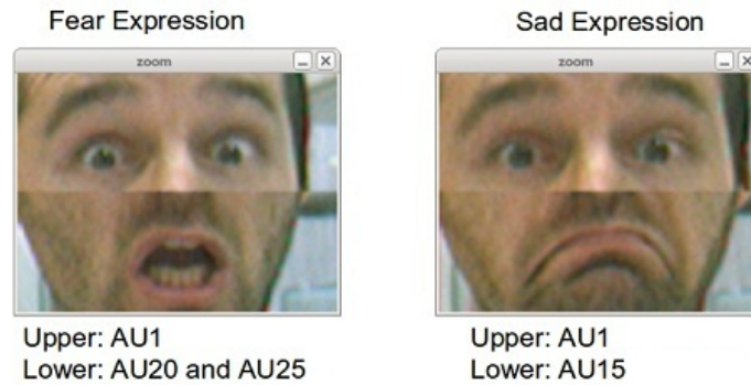
Figure 2.6: Sample results of our method for image face feature extraction. Left image presents a fear expression; right image presents a sad expression. The face is separated in upper and lower face. The nose part is discarded. The detected AUs are presented under each of the respective images.
