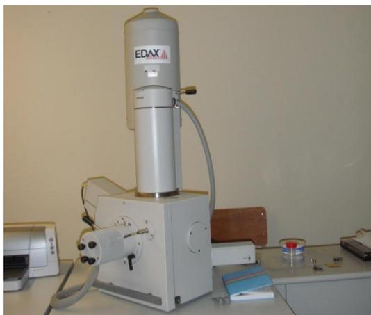
Figura 40 – Scanning electron microscope (SEM)
