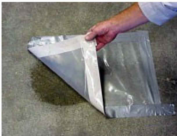
Figura 4.6 - Plastic Sheet Test [33].
