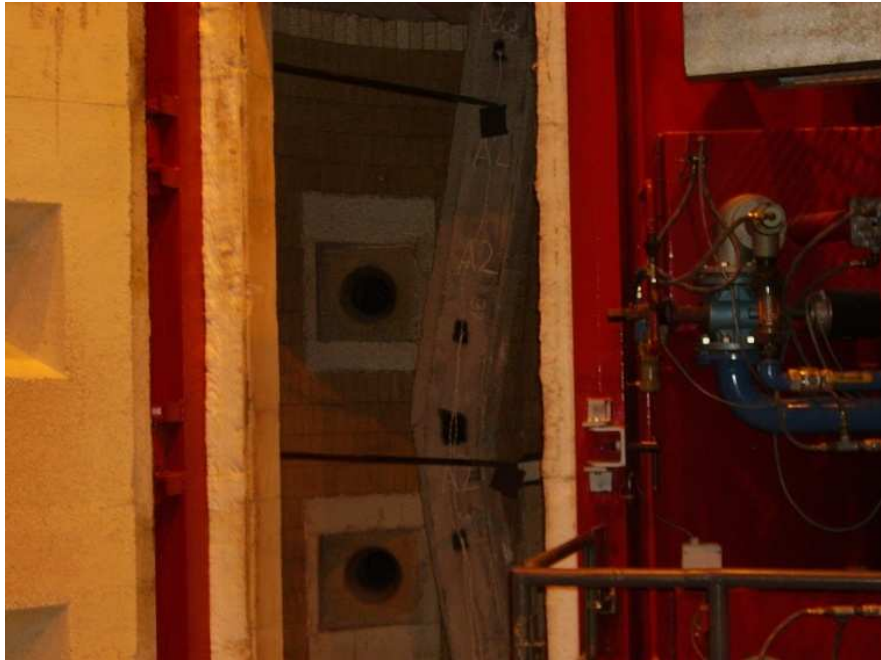
Figure 5.41 – View of the deformed shape of column BAM-CSC200-K11-L70 after test
