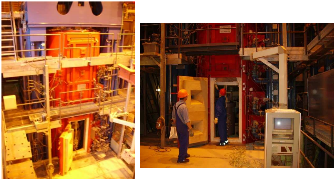
Figure 5.5 – View of the vertical furnace for testing columns
