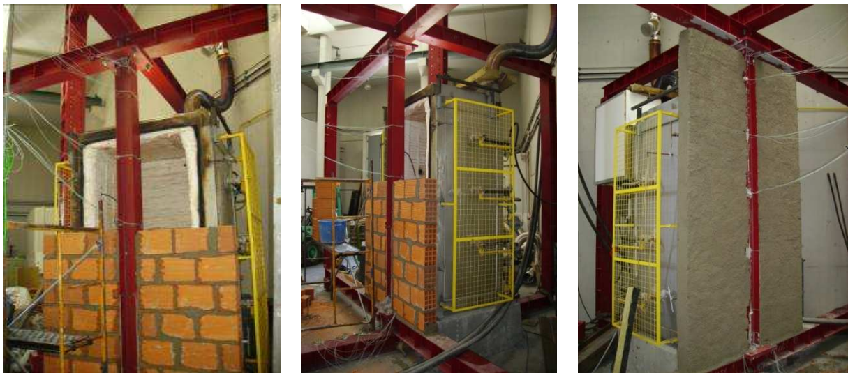
Figure 4.15 – a) Construction of the test model b) Column embedded on a wall c) Lateral view of the experimental system.
