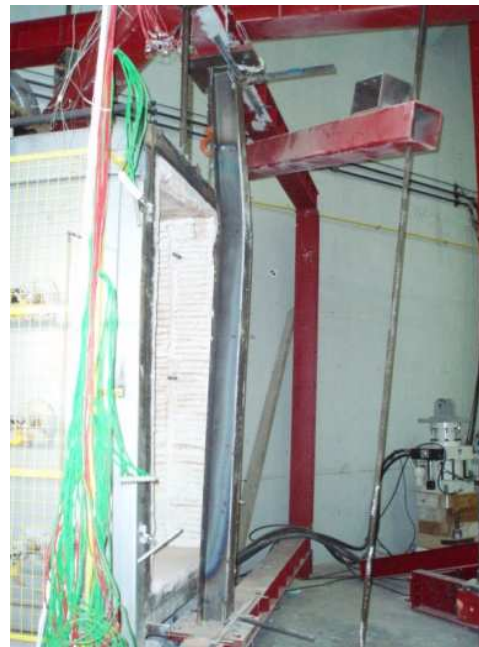
Figure 4.53 - Column E02 after test - web perpendicular to wall – wall thickness 140mm - HEA 160
