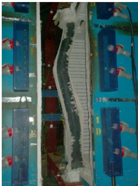
Figure 4.58 - Columns after test a) column of test CSC200-K128-L30 b) column CSC160-K13-L30
