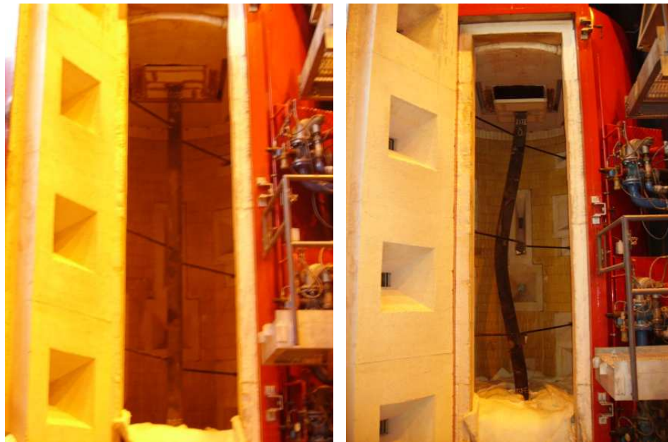
Figure 5.35 – Views of column of test BAM-SC140-K47-L70 before and after test
