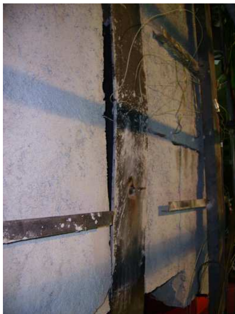
Figure 4.53 - Column E02 after test - web perpendicular to wall – wall thickness 140mm - HEA 160
