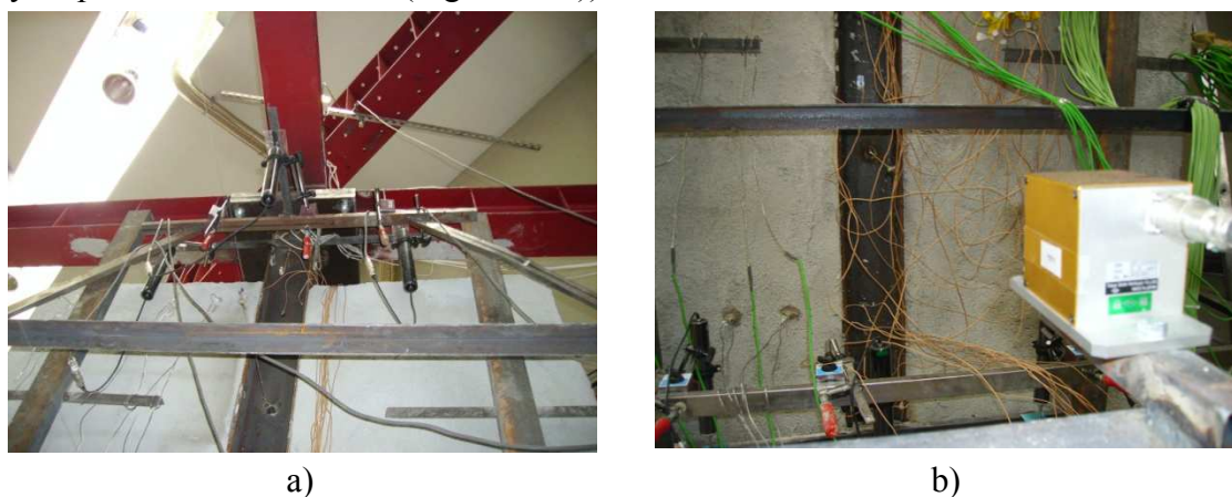
Figure 4.3 - Displacement transducers a) at bottom of the column b) at top of the column
