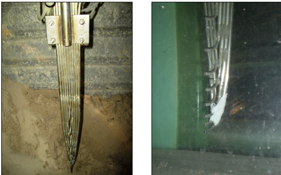
Figure 3.12 – Probe of Transverse Suction System .
