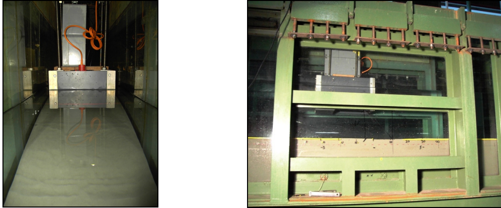
Figure 3.6 – Laser Bed Level Profiler in the LOWT (front view and side view).
