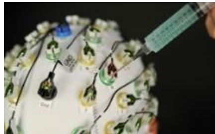
Fig. 4.16 - Placement of gel in the electrodes. If the electrode impedance is above 20 K \Omega , the electrode led turns red. If the value of impedance is acceptable (below 15 K \Omega ), the colour of the led turns green (Brain Products GmbH, 2009).
