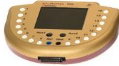
Fig. 4.2 - V-amp amplifier from BrainProducts (Brain Products GmbH, 2009).
