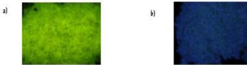
Figure 19 – Solid CL viewed by FM with two different excitation wavelengths filters: a) 470-495nm; b) 360-370nm.
