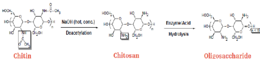
Figure 7 – Structure of chitin and the reactions that lead to the chitosan and to the corresponding oligosaccharide. (Adapted from Sigma-Aldrich products section).
