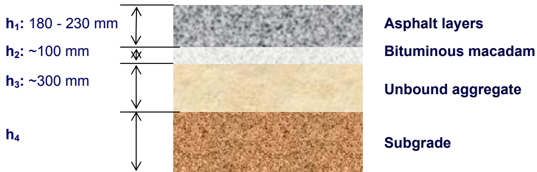
Figure 7.1 – Pavement structure sketch
