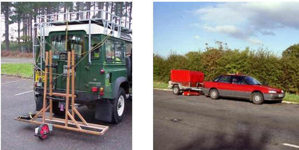
Figure 4.2 - Examples of dipole close air coupled antennas used for survey at traffic speed [FORMAT; 2004]
