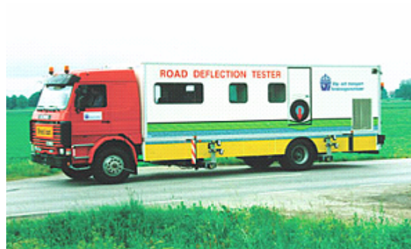
Figure 3.11 - The Swedish Road Deflection Tester
