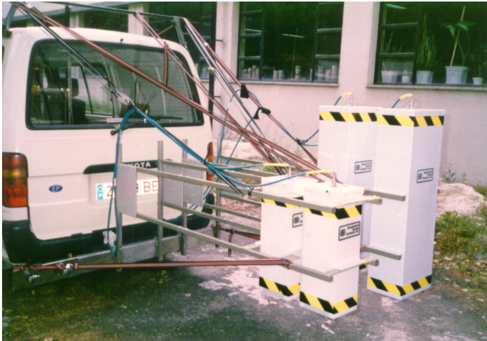
Figure 4.5 – LNEC’s equipment – initial structure: suspension system
