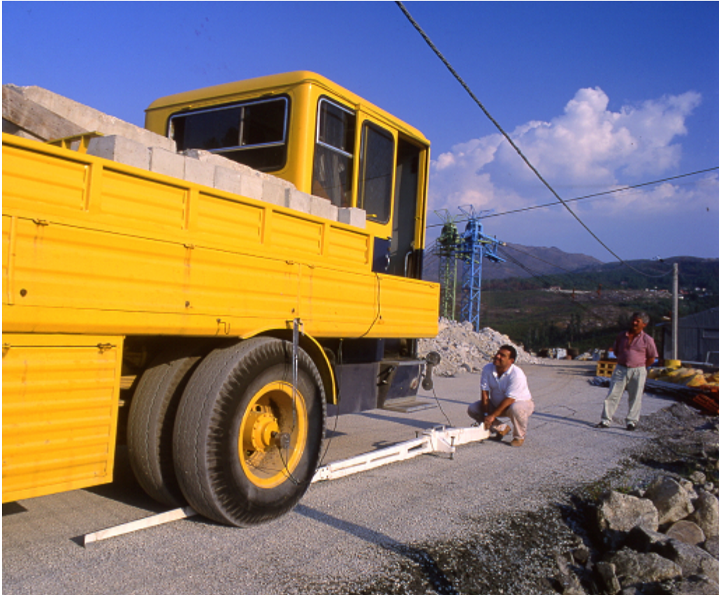
Figure 3.7 – “LNEC deflectograph” during tests
