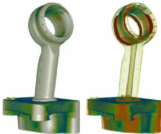
Figure 2.22: Three-dimensional reconstructions of parts of a fuel injector device. Metallic components can be extracted or suppressed by image processing. After [And09].
