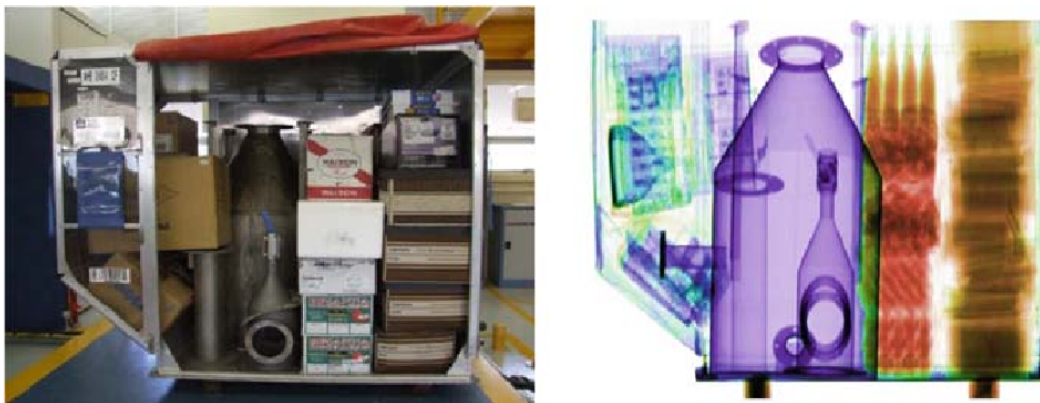
Figure 2.23: Neutron imaging applied to homeland security. Optical picture (left) and a neutron image of an aircraft container (right). After [And09].
