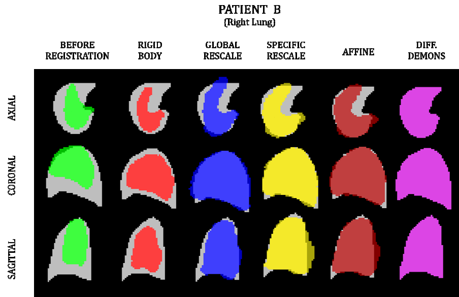
Figure 21 Overlay of reference image (gray) and moving image of patient B (right lung) before registration process (green) and after registration: rigid body algorithm (red), global rescale (blue), specific rescale (yellow), affine (brown) and diffeomorphic demons (pink).
