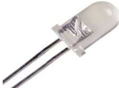
Figure 4-13: LED used as light source in the polarimeter [AD58]
