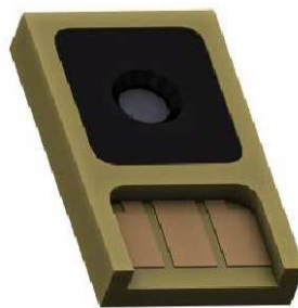
Figure 4-1: ISFET Chip OII1 [AD68]
