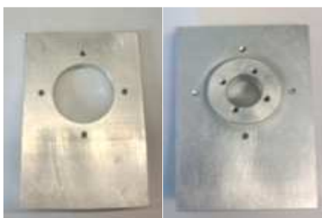
Figure 4-12: Optical mounts used in the polarimeter: a) Standard mount; b) Analyser mount
