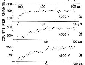
Fig. 8. Distributions of the time intervals between successive streamers. The time ranges of the time to amplitude converter unit are indicated. For 800  $\mu s$  time range linear fits are displayed.
