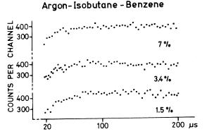
Fig. 9. Influence of the benzene concentration on the distribution of the time intervals between successive streamers for 4300 volts.
