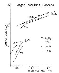
Fig. 4. The average amplitudes of the current pulses from the chamber for the different argon-isobutane-benzene mixtures used.
