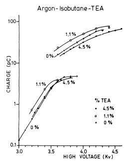
Fig. 1. A comparison of charge characteristics of the chamber for various argon-isobutane-TEA mixtures.
