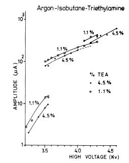
Fig. 3. The average amplitudes of the current pulses from the chamber for two different argon-isobutane-TEA mixtures.
