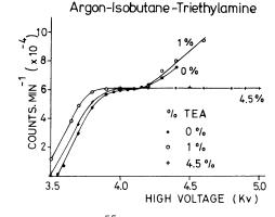
Fig. 6. Counting rate (<sup>55</sup>Fe source) versus high voltage for various argon-isobutane-TEA mixtures.
