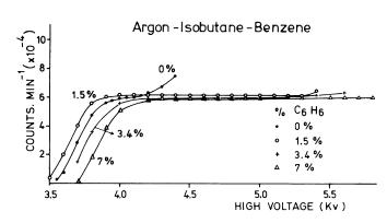
Fig. 7. Counting rate (<sup>55</sup>Fe source) versus high voltage for various argon-isobutane-benzene mixtures.
