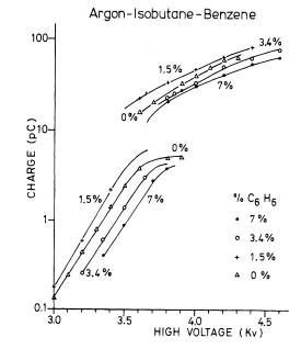
Fig. 2. A comparison of charge characteristics of the chamber for various argon-isobutane-benzene mixtures.
