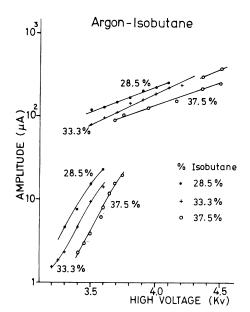
Fig. 5. The average amplitudes of the current pulses from the chamber for various concentrations of argon and isobutane.
