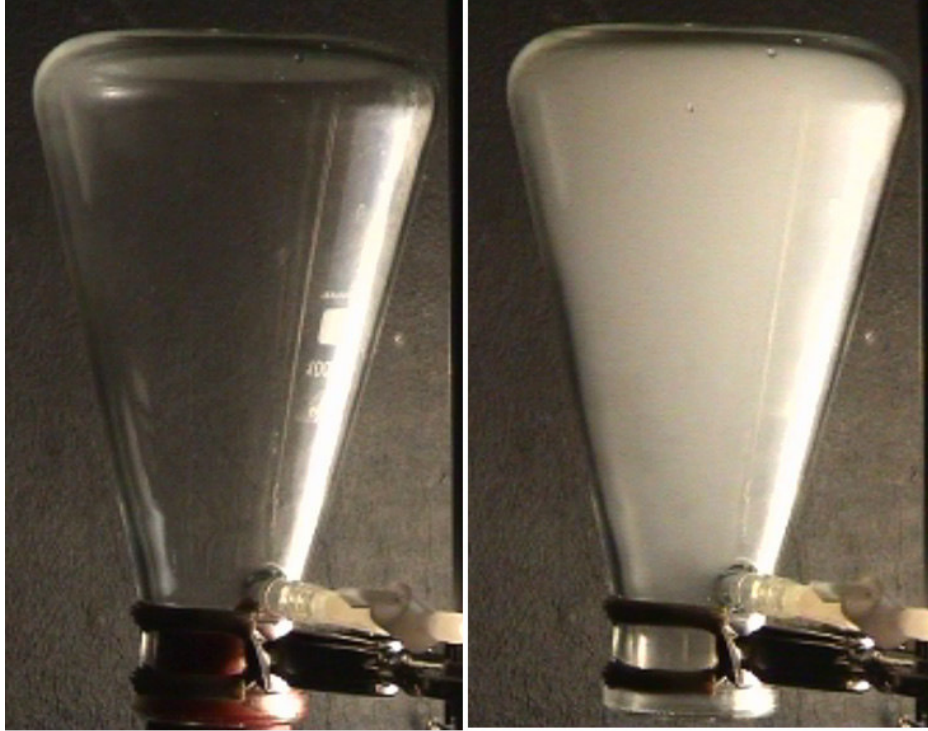
Figure 2: Fog in a bottle. The pressure is increased inside the bottle. When the cork flies apart from the bottle, the abrupt decrease of the pressure originates a cloud. The experiment works better if few drops of water are placed inside the flask (as suggested by Coop, see footnote 13).
