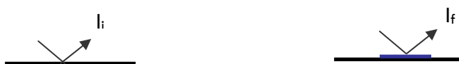
Figure 8.5 - Schematic representation of the light beams involved in the optical density measurement.
