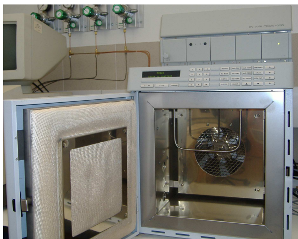
Figure 7.5 – Gas chromatograph DANI GC1000, used in the IGC measurements.
