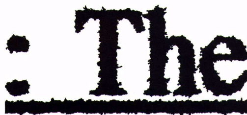
Figure 8.8 – Exemplification of feathering of a printed area.
