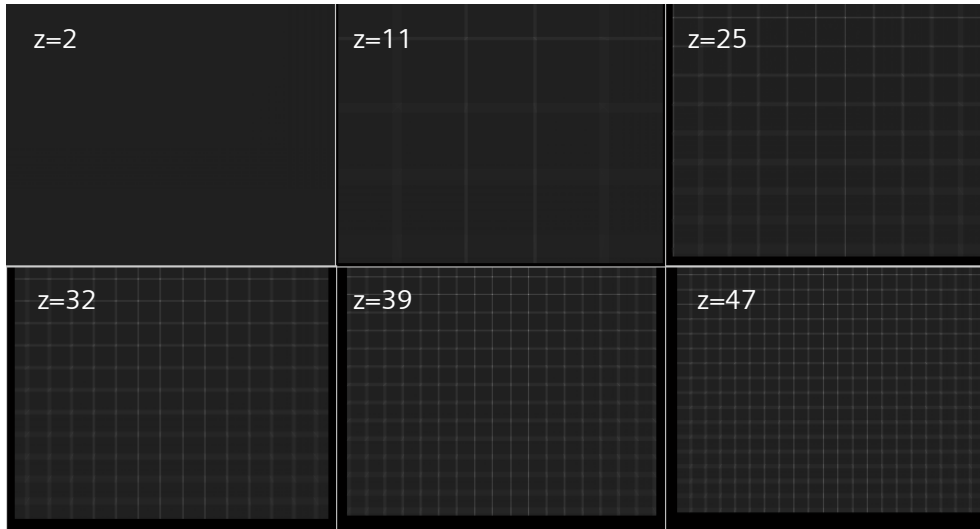
Figure 7.10 Slices 2, 11, 25, 32, 39 and 47 from a volume resultant from the back projection of a uniform image, using the system matrix constructed.
