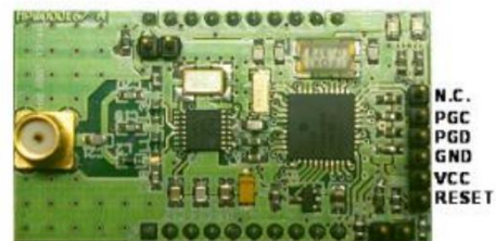
FIGURE 6.9: Connecting to the type of programming the ICD2 [30]
