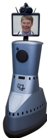
Figure 12 - Robot's panoramic Virtually There visualization system.
