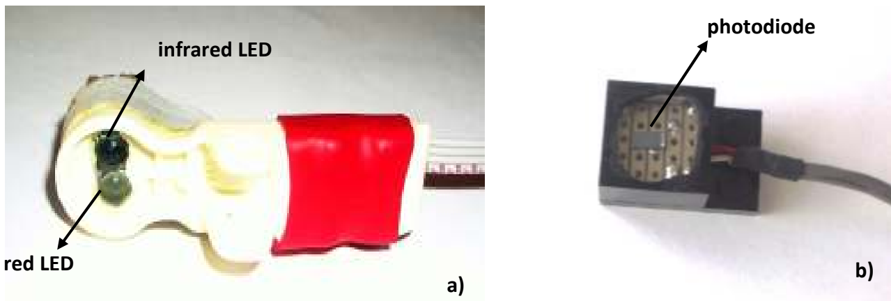
Figure 28. Arms of the Oximeter Probe Prototype. 28a) – arm containing the red and the infrared LEDs ; 28b) - arm containing the photodiode
