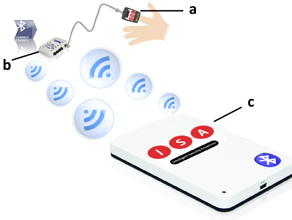
Figure 26. System Architecture; a - oximeter probe; b – acquisition module; c – processing module
