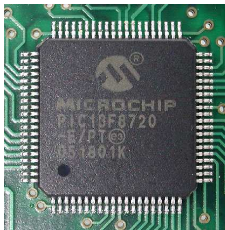
Figure 6 - A PIC 18F8720 microcontroller in an 80-pin TQFP package.
