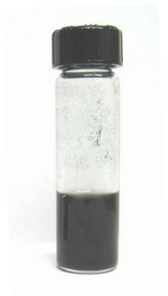
Figure 56: SWNTs suspended in sodium cholate. A characteristic dark-colored aqueous suspension was obtained as result of this sonication process (Palwai 2007).
