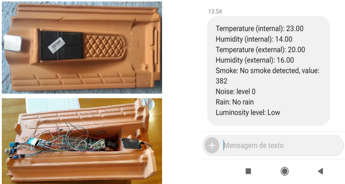
Figure 2. Smart Roof Tile Prototype and Interaction Example (SMS)
