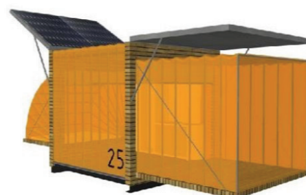
Shelter with materials for DESERT and SAVANA ZONES modified for coupling with other shelters
