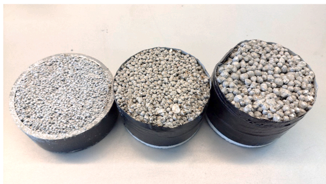
Fig. 2. Example of test specimens prepared with each of the size classes of expanded clay used in this study.
