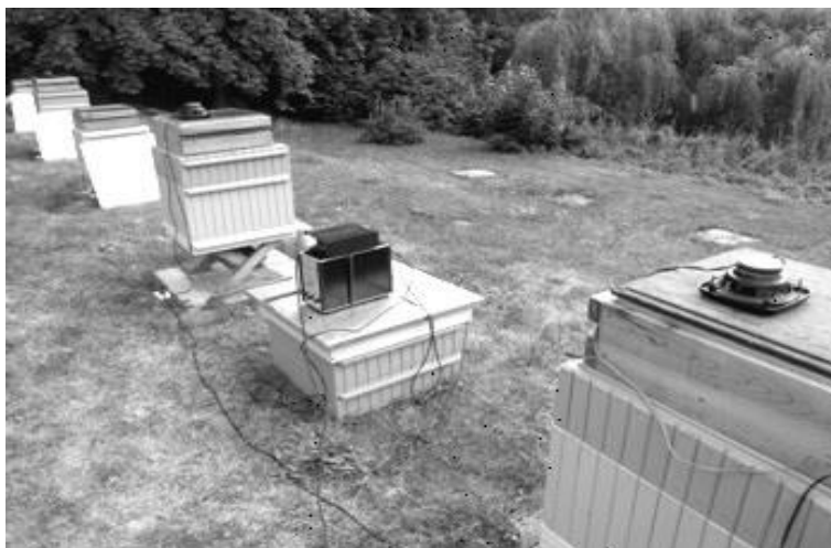
Figure 177. A set of equipment used for venom collection using combined electrical and sound stimulus.
