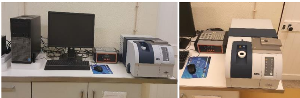
Figure 22. BRUKER spectrometer operated with the OPUS®, version 7.5.18 (Bruker Optic, Germany) software in reflectance mode.
