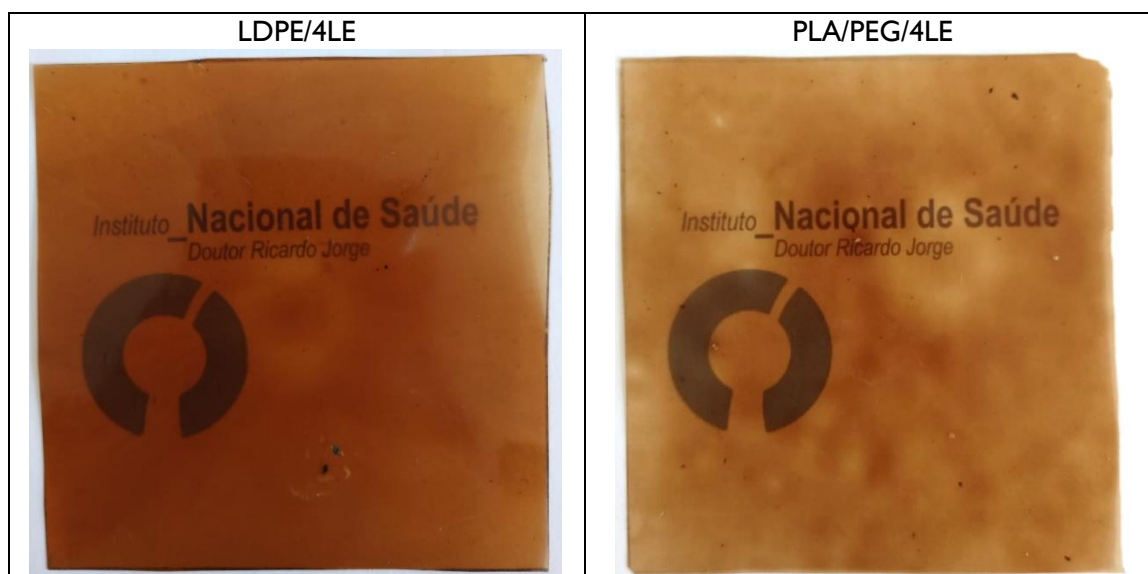
Figure VII.1. Active (LDPE/4LE and PLA/PEG/4LE) films over the Portuguese National Institute of Health logo.
