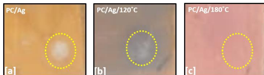
Figure 7. Pictures of the scratch-tested areas of the sample: (a) PC/Ag; (b) PC/Ag/120 °C; (c) PC/Ag/180 °C. Yellow dotted circles were added around the tested zones to facilitate interpretation.
