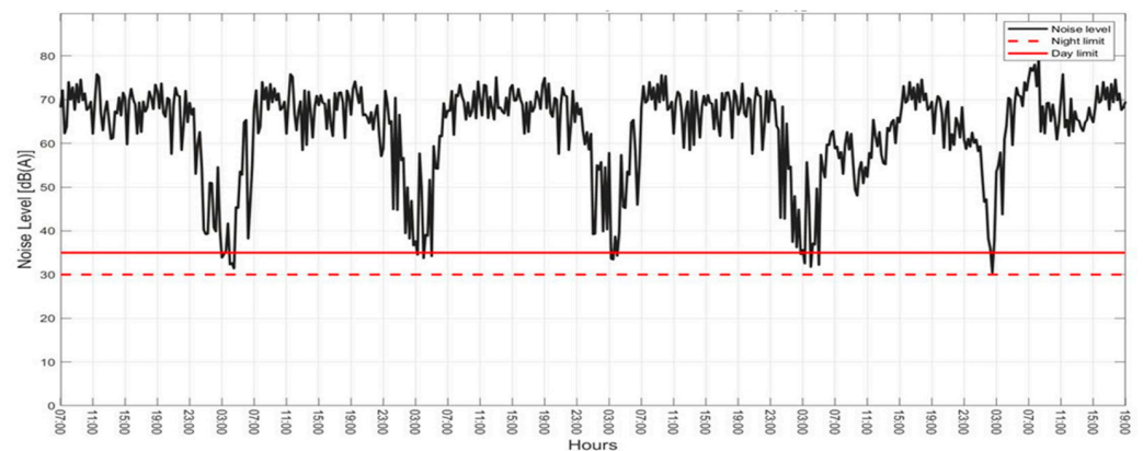
Figure 6. Shows the weekly noise level in the CH. Note: The middle line represents 35 dBA, the WHO-recommended noise level during the day, while the lowest line (dash line) represents 30 dBA, the WHO recommendation during the night. The noise produced by this equipment greatly surpasses the acceptable noise levels in the ICU.
