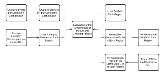
Figure 4. Evaluation of the impact on the electrical grid.
